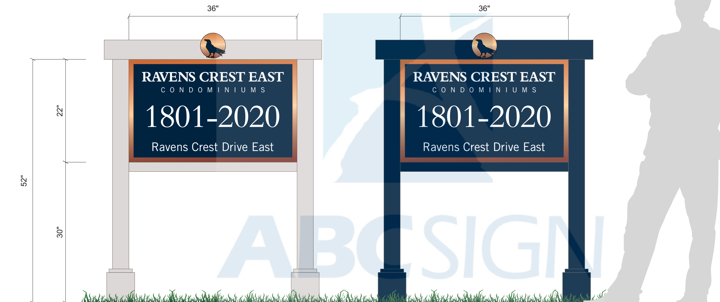
Typical Identity Sign - Double Face Scale: 1" = 1'-0"
